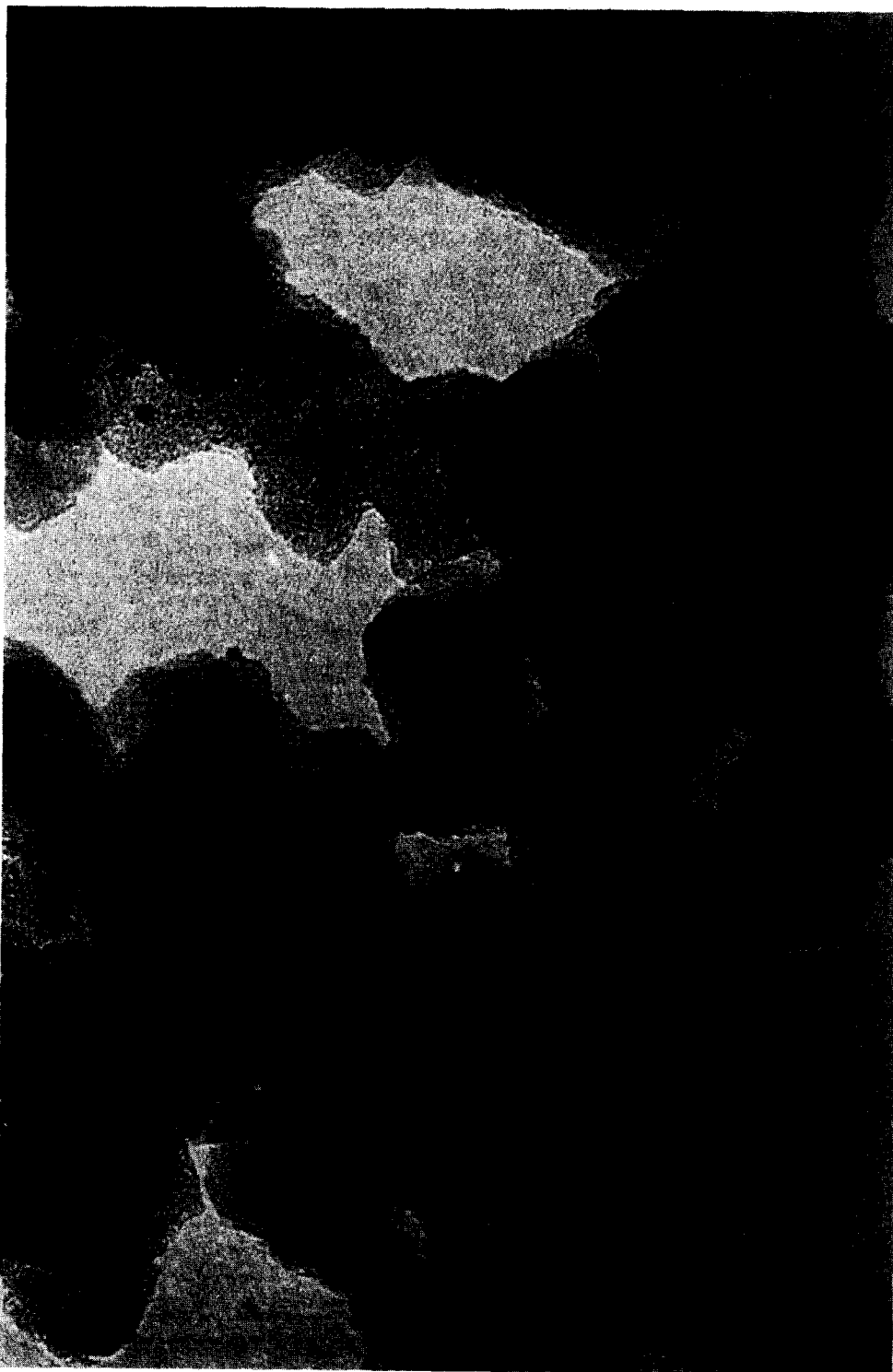
FIG. 2. Electron micrograph of the amine-modified silica catalyst containing Rh (sample MA1) after H_2 treatments in infrared experiments. Rh crystallites are clearly visible.
